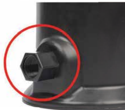
Hexagonal Inlet/Outlet fittings: Keyed through meter box wall, preventing rotation and internal leaks at time of installation
