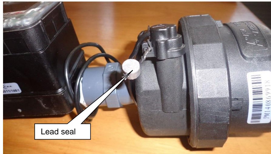
Illustration 6 Photograph showing the application of the protective mark on the pulse output
